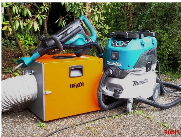
Figure 8: Sucked off hand-held tools (here a demolition hammer), construction dust collector and air cleaner. These minimum equipment with low-dust techniques does not even cost 3,000 euro
