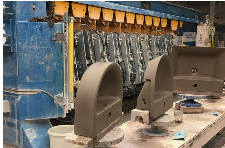
Medium pressure casting with resin moulds
